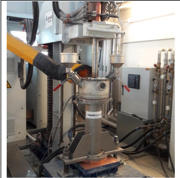
Fig. 1: Laboratory-ESR-plant with the new mould in operation under protective atmosphere (Source: Univ. of Appl. Sciences Upper Austria)
