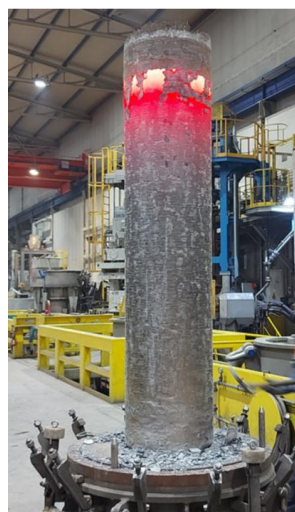
Figure 1: Pressure ESR ingot (voestalpine Boehler Edelstahl)
