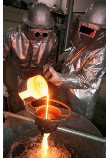
Water granulation in melting laboratory of FEHS – Building Materials Institute
