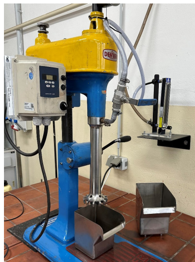
Figure 2. Laboratory Denver D-12 flotation machine (with 1.2 and 2.4 L cells).
