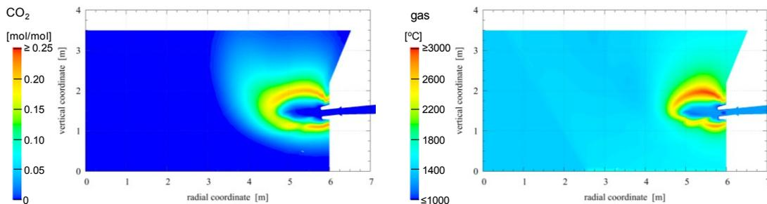
Figure 7: Left: Contours of CO<sub>2</sub> mole fraction. Right: Gas-phase temperature field.
