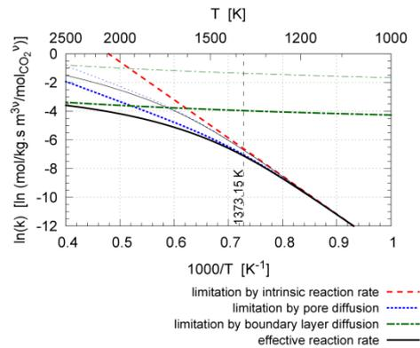
Figure 4: Reaction rates at mean concentration in the coke bed, bold lines: exp. 2, light lines: exp. 5.
