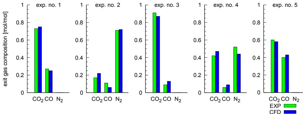
Figure 6: Product gas composition, comparison of exp. data and CFD results (major gas constituents).
