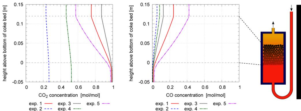
Figure 5: Profiles of CO<sub>2</sub> and CO mole fractions along the coke bed.
