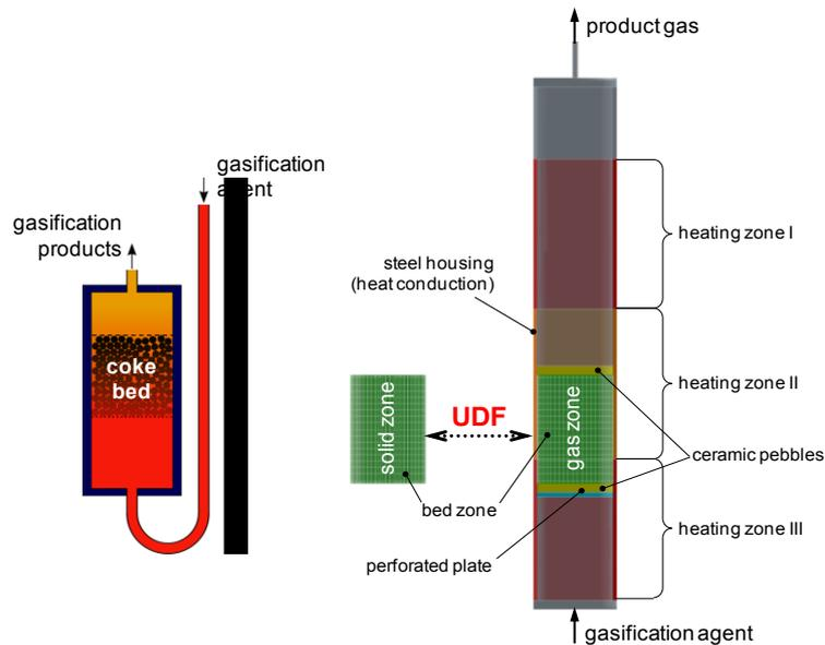
Figure 2: Schematic illustration of the NSC-test (left) and its implementation in the CFD-model (right).
