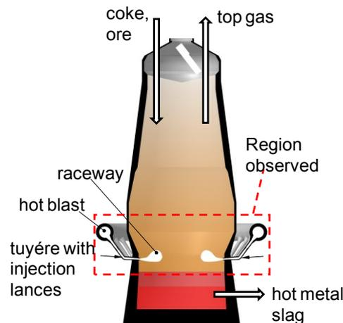
Figure 1: Scheme of the blast furnace, highlighting the zone under investigation (Maier et al., 2013).
