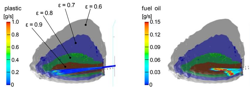
Figure 8: Tracks of injected auxiliary reducing agents, coloured by mass release rates. Iso-surfaces, coloured by local coke bed void fraction  $\varepsilon$ , defining the shape of the raceway cavity.
