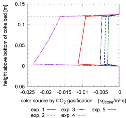
Figure 3: Vertical profile of coke consumption rates due to the solution loss reaction, conditions as listed in Table 1.
