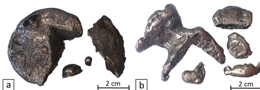
Figure B2. Representative samples of the alloy after pyrometallurgical treatment in the InduMelt reactor: a.) LFP, b.) NMC811
