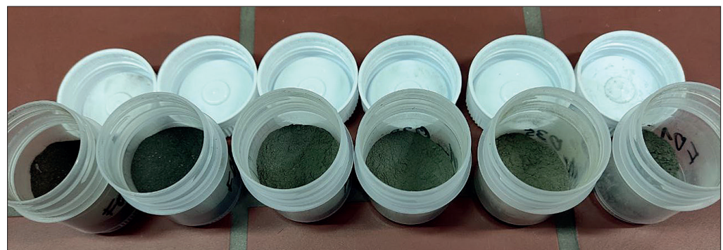
Fig. 11: Prepared samples of secondary slags with rising iron addition (from left to right)
