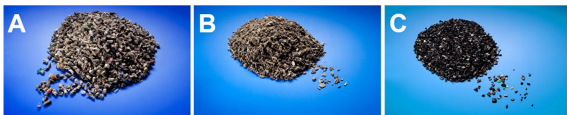
Fig. 4 Waste plastics used at voestalpine Stahl (A = pellets, B = agglomerate, C = granulate) [22]
