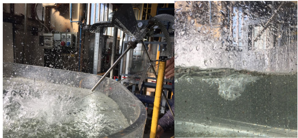
Fig. 12 Image of the EAF water model testing with injection of polymers and penetration into the bath [8]
