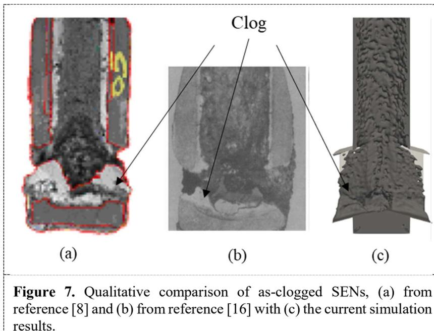
**Figure 7.** Qualitative comparison of as-clogged SENs, (a) from reference [8] and (b) from reference [16] with (c) the current simulation results.
