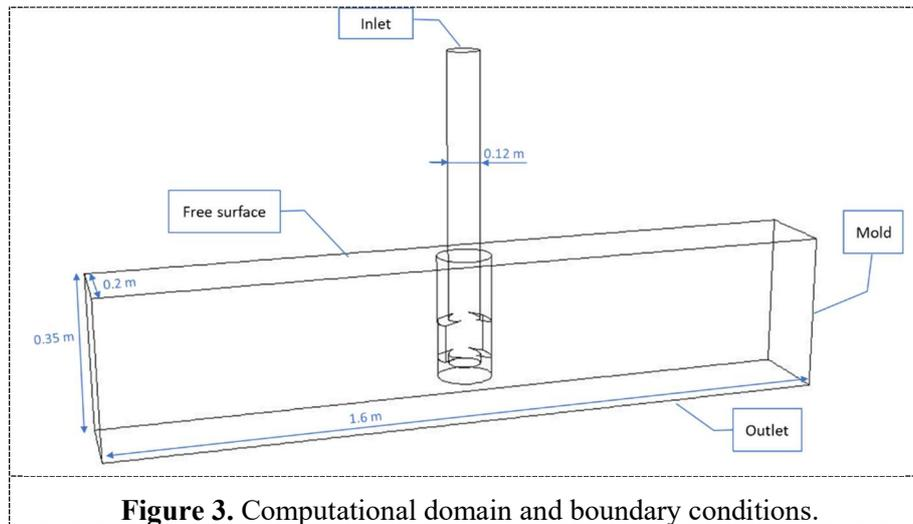
**Figure 3.** Computational domain and boundary conditions.
