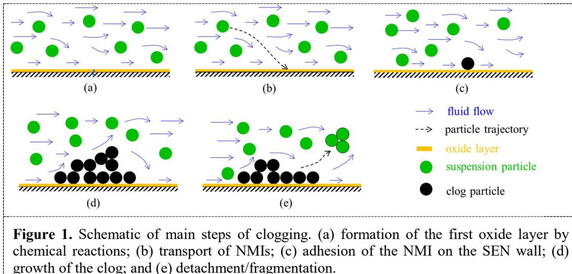
**Figure 1.** Schematic of main steps of clogging. (a) formation of the first oxide layer by chemical reactions; (b) transport of NMIs; (c) adhesion of the NMI on the SEN wall; (d) growth of the clog; and (e) detachment/fragmentation.
