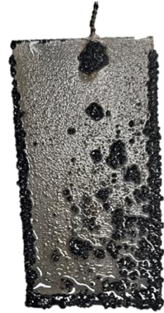
Figure 2: Deposition of zinc onto the electrode.
