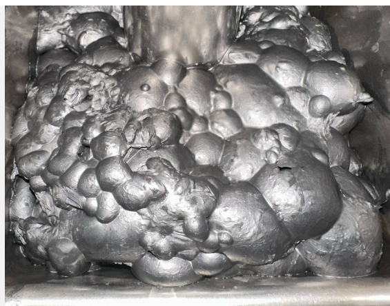
Figure 1: Froth flotation of black mass for the recovery and enrichment of graphite in the froth product (© UVR-FIA).
