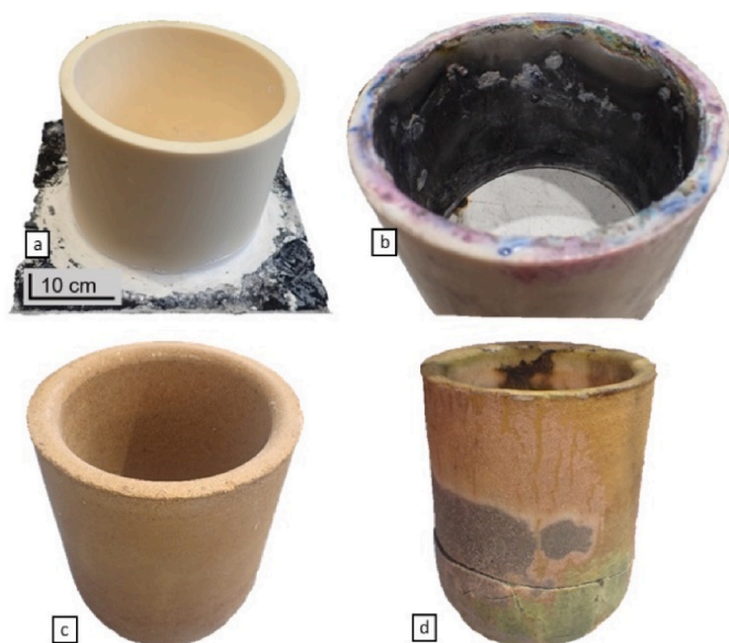
Fig. 5. Crucibles before (a,c) and after (b, d) InduMelt trials; b): \text{Al}_2\text{O}_3 crucible with heavy corrosion signs ( https://www.mdpi.com/2227-9717/9/1/84 ); d): \text{MgO} crucible with diffusion signs and cracks at the bottom (dimensions as seen within Fig. 3).
